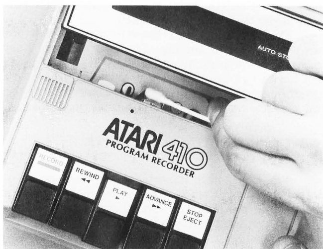
FIGURE 5.1. Cleaning the recorder heads.
