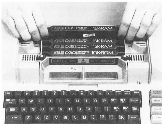
FIGURE 1.2. The 800 computer with its cover removed revealing plug-in 16K memory cartridges and a 10K ROM cartridge.
